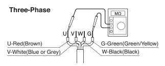
**Note:** The insulation resistance reference value of  $20M \Omega$  minimum is based on a new or repaired pump. For reference values of a pump that has already been put into operation, refer to section "7. Maintenance and Inspection" of this manual.
