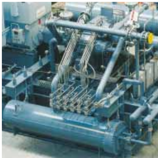
CO compressor (Atlas Copco) at Alkos, Yochon/Korea, with a Burgmann DGS2/49 gas seal. p_1 = 2.2 \dots 28 bar a; n = 21,700/34,800 min -1 ; medium: carbon monoxide.
