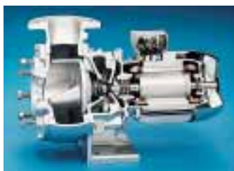
Sewage block pump (Herborner, Type Unipump) for pumping contaminated fluids containing solids up to 80 mm with a double mechanical seal (MG1/M3S35 on the product side) in tandem arrangement. Quenching fluid: oil.
