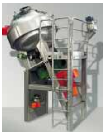
Spherical dryer (Rosenmund Gueda) for the production of pharmaceutical powders, with Burgmann HSMR5L-D (main and chopper shafts).
