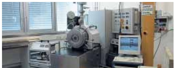
High-speed test rig for small-diameter seals and clearance seals
