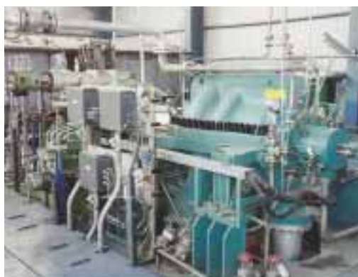
Ethylene compressor (Demag Delaval) at the Yanshan Petrochemical Plant (China). Sealed with Burgmann PDGS1/195, elastomer-free. p_1 = 3.8 bara; t = -80 °C; v_g = 100 m/s; n = 7,830 min -1 .
