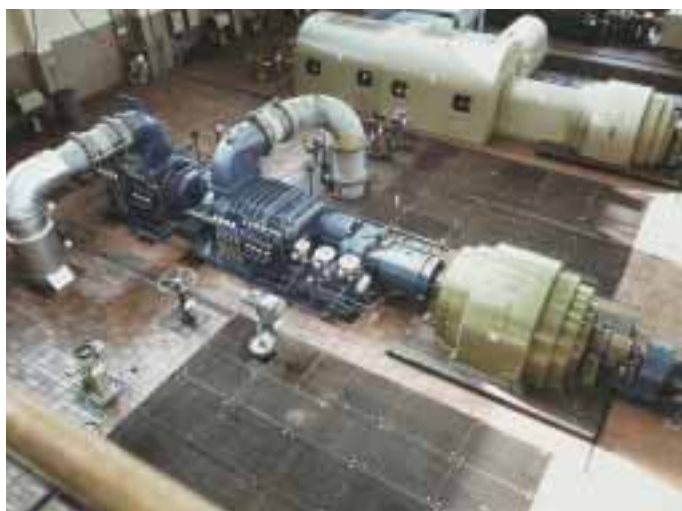
Ethylene compressor (Demag Delaval) at the Yanshan Petrochemical Plant (China). Sealed with Burgmann PDGS1/195, elastomer-free. p_1 = 3.8 bara; t = -80 °C; v_g = 100 m/s; n = 7,830 min -1 .
