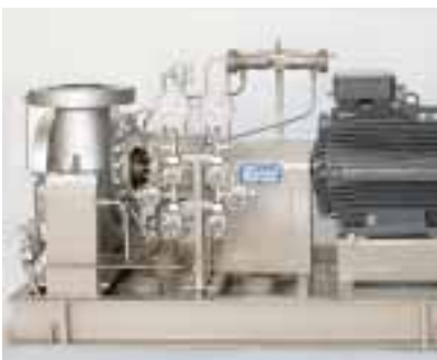
Boiler circulation pump (PRNR, ENSIVAL) with SHV1/57-EF1 seal and WED20 heat exchanger. ( t = 325\text{ }^{\circ}\text{C} ; H = 122.95\text{ kg/cm}^2 ; p = 120.5\text{ bar} )
