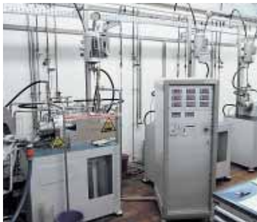
High-pressure test rigs for performance-testing face materials
