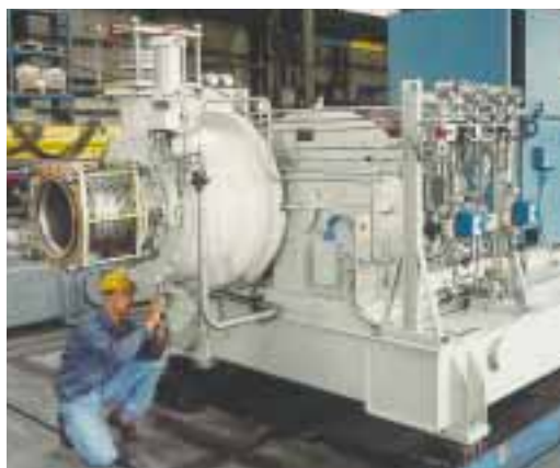
Ammonia compressor (Sulzer-Turbo) at Norsk Hydro, Trinidad. The compressor system was equipped with a Burgmann DGS, independent of the direction of rotation, in a tandem arrangement with internal intermediate labyrinth and a Burgmann buffer gas system. The system has been running without trouble since 1995. d_1 = 100 mm; p = 4.7 bar a; n = 15,850 min -1 ; medium: ammonia.
