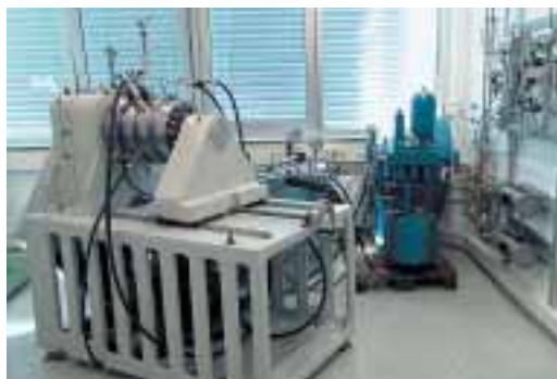
High-pressure test rig for high speed running seals, with separate control desk (photo at right)
