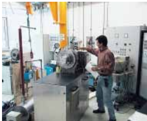
Basic test stand for high speed running gas seals and segmental radial seals for turbocompressors and drive mechanisms
