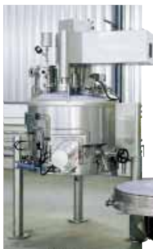
◀ Filter dryer (Rosenmund Gueda) with Burgmann M451 KL(T)-D and AGS451 KL-D ( p_1 = vacuum ... 6 bar; t_1 = -20 ... 200 °C; n = 5 ... 50 min -1 ; axial movement) 100 ... 700 mm)
