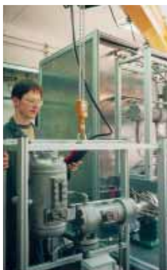
Test facility for qualifying mechanical seals to API standard
