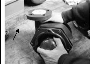
Figure 8-23: Wet end assembly
