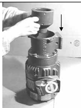
Figure 8-5: Assembly of outer drive
