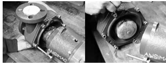
Figure 8-25: Assembly of wet end to motor drive
