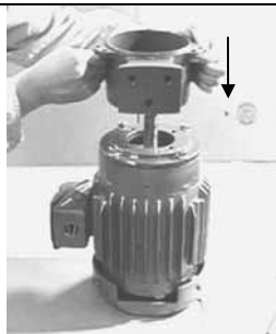
Figure 8-3: Assembly of close coupled bracket
