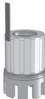
Figure 6.26 – Assemble Magnet Segments
