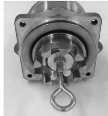
Figure – 6.31 Rotor Assembly in Place
