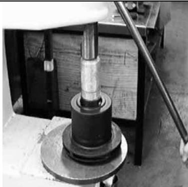
Fig.8-4: Insert Bushing into Impeller with Arbor Press
