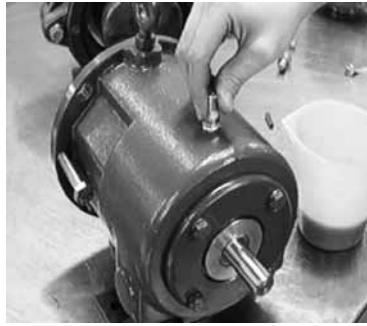
Fig. 12-21: Remove Breathing Tube
