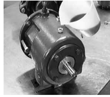
Fig. 12-22: Fill Bearing Frame with Oil
