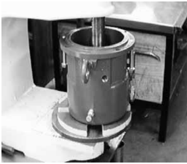
Fig. 12-16: Install Labyrinth Seal into Cavity
