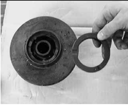
Fig.8-7: Press-Fit Mouth Ring into Impeller
