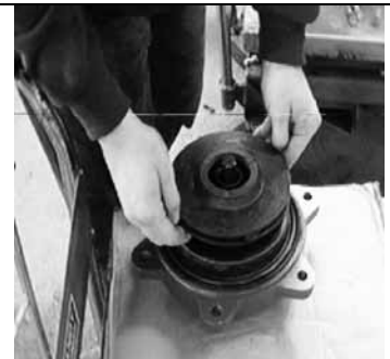
Fig. 7-10: Remove Impeller from Containment Shell
