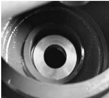
Fig. 12-17: Labyrinth Seal in Cavity
