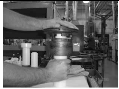
Figure 7-14: Separation of the impeller and inner drive
