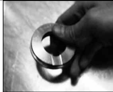
Fig. 11-15: Labyrinth Seal w/ Port at 6 o'clock
