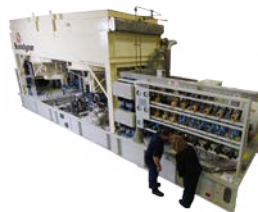
Sundyne BMC-337 is a single-stage centrifugal compressor
