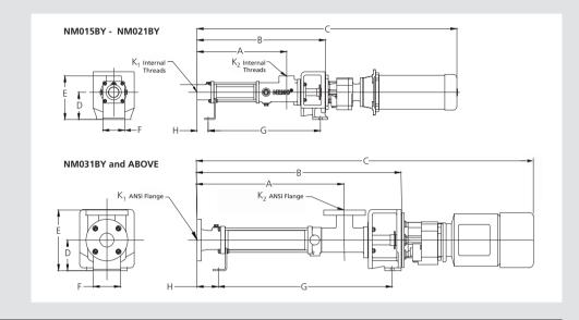
Flow rate up to 1800 GPM / 410 m³/h Pressures up to 360 psi / 24 bar
