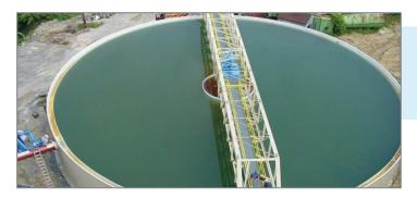
The WesTech HiFlo<sup>TM</sup> thickener achieves significantly more throughput than a conventional thickener of similar size while significantly reducing water consumption and substantially saving on flocculant costs.
