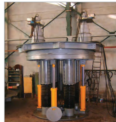
Cage Drive with Hydraulic Lift
