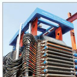
The **WesTech Tower Press Filter** provides ultra-low moisture content performance compared to a traditional atmosphere-dependent vacuum filter. It eliminates short-circuiting by stacking the filter plates vertically, allowing feed slurry to flow evenly throughout.
