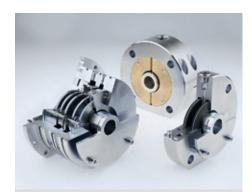
Carbon floating ring seals are supplied as maintenance free compact labyrinth cartridge seals with low leakage. The floating self-adjusting sealing rings provide radial sealing on the shaft with a very small gap. The seal requires no additional lubrication, and it is designed for dry running. Besides pure gas, carbon floating ring seals are also suitable for Atex applications, toxic media, media containing solids, flue gas, dust, powder, vapor, liquid mist, oil mist and penetrating oil.
