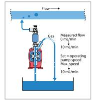
After the gas has been purged, the EFS sensor will begin to measure flow. Feedback from the sensor controls the pump, slowing it back down so the flow rate meets the set value
