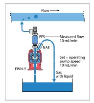
The auto air vent valve bleeds gas and liquid out of the pump chamber. However, pump output is maintained due to the feedback control from the flow sensor.
