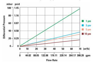
Note: the inner diameter of the filter element and the filter housing in/outlet is the limited factor
