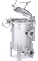
MAXILINE & PROLINE multi-bag filter housings are for high-volume applications demanding frequent filter bag change-outs. Available in a wide variety of configurations with 4 to 24 filter bags per housing. Options include: various input/output positions and sizes, material choices and closure designs.
