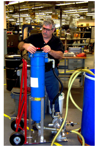
Eaton's FLOWLINE filter housing with their high performance DURAGAF™ filter bag during the coolant filtration process.
