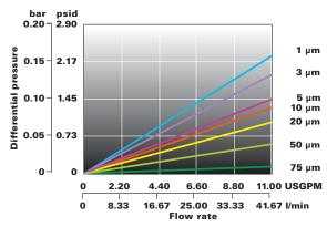
\* For liquids other than water, multiply pressure drop by fluid viscosity in centipoise.
