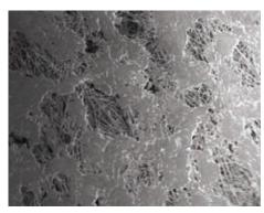
Surface of a MAX-LOAD pleated filter bag
