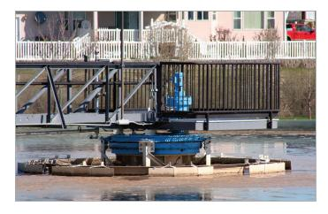
WesTech **Drive Units** are specifically engineered for the high torque requirements of minerals thickeners. They are designed with a direct in-line high efficiency speed reducer and motor stack as well as a durable precision bearing. State-of-the-art torque protection and rake lifting capability ensure an unrivaled customized design for each application.
