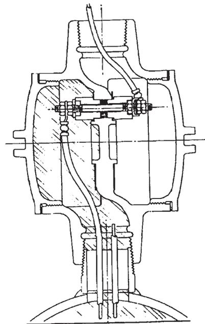
Figure 2-14. Leakproof Junction Box
