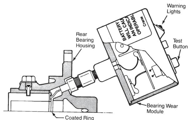
Figure 2-15. Bearing Wear Detector
