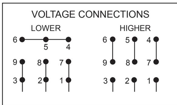
Figure 2-2. 3-Phase Dual-Voltage Connections
