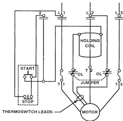
Figure 2-3. Wiring Diagram 230/460 Volt, 3 Phase
