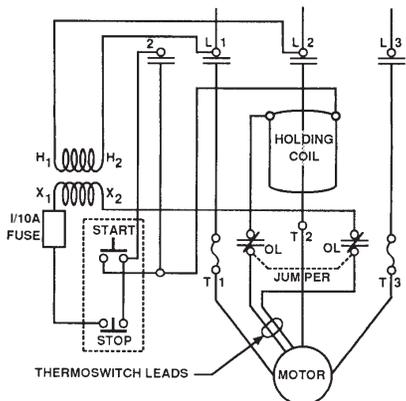
Figure 2-4. Wiring Diagram 575 Volt, 3 Phase
