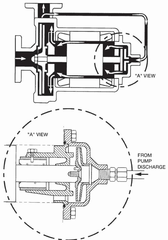
Figure 2-8. Pressurized Recirculation
