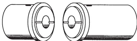
Figure 1-4. Bearings - Series G Chempump Sleeved Type
