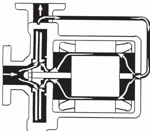
Figure 1-1. Series G Chempump Schematic Diagram, Standard Circulation Single Stage
