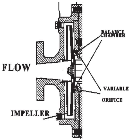
Figure 1-8. Automatic Thrust Balance, Single Ring
