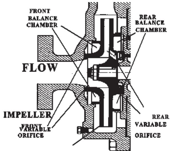
Figure 1-9. Automatic Thrust Balance, Double Ring.
