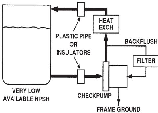
Figure 2.9 Back Flush Installation with Electrical Isolation
