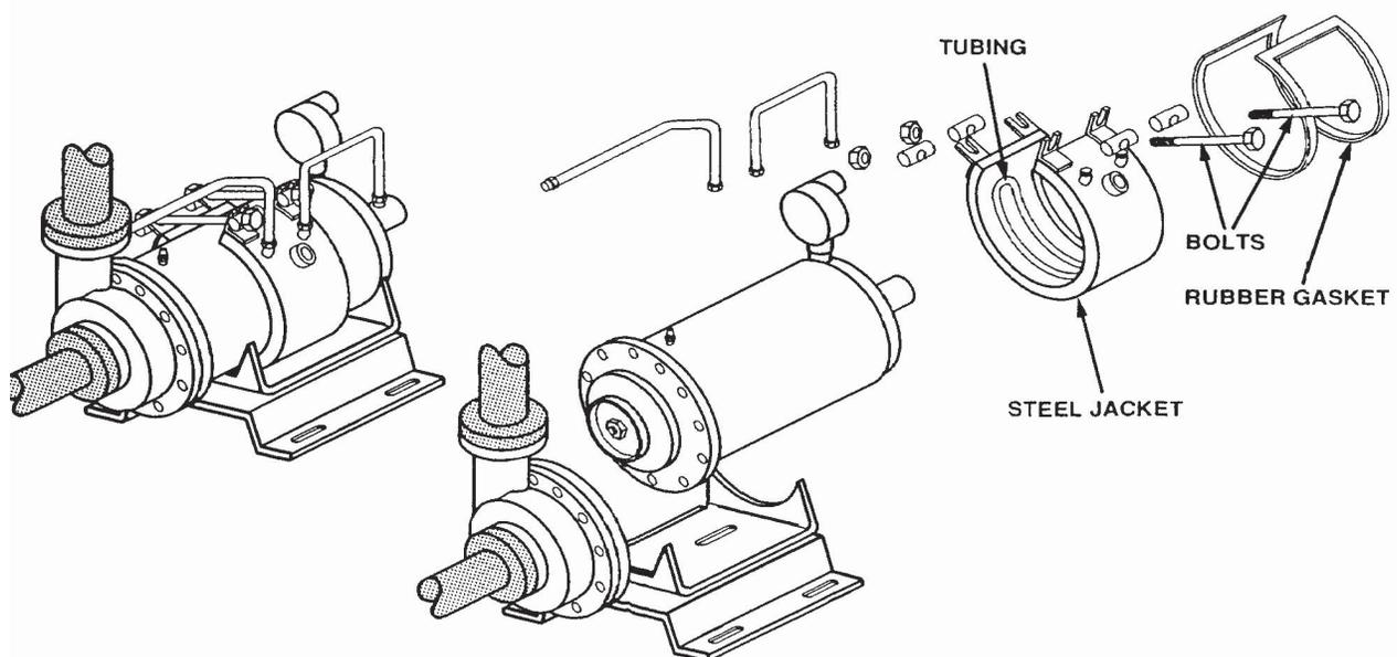
Figure 2-11. Removable Heat Exchanger
