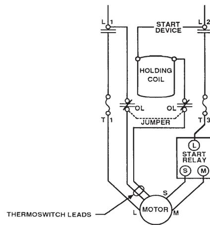
Figure 2-5. Wiring Diagram 115/230 Volt, 1 Phase
