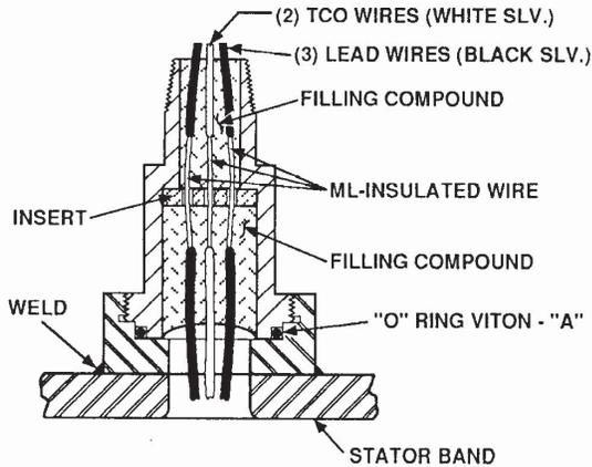
Figure 2-13. High Pressure Lead Connector
