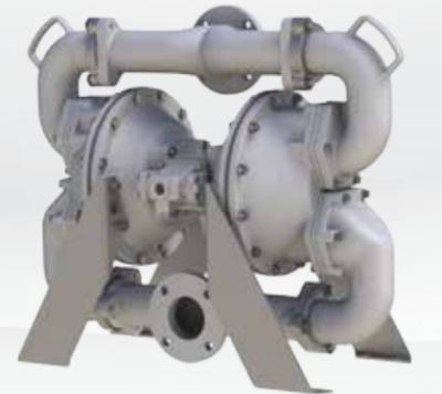
**SOLIDS HANDLING** Up to 3" (75 mm)   **MAX FLOW** 260 GPM (984 LPM)   **MAX PRESSURE** 125 psi (8.6 bar)   **DISPLACEMENT** 1.5 gallon (5.7 liter)
