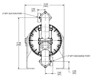
2" NPT(F) Suction and Discharge • ¾" NPT(F) Air Inlet Port • ¾" NPT(F) Air Exhaust Port (not shown)
