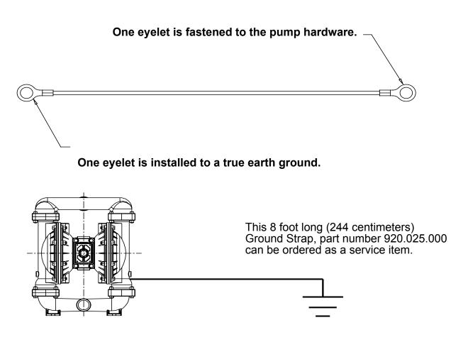
To reduce the risk of static electrical sparking, this pump must be grounded. Check the local electrical code for detailed grounding instruction and the type of equipment required, or in the absence of local codes, an industry or nationally recognized code having jurisdiction over specific installations.
