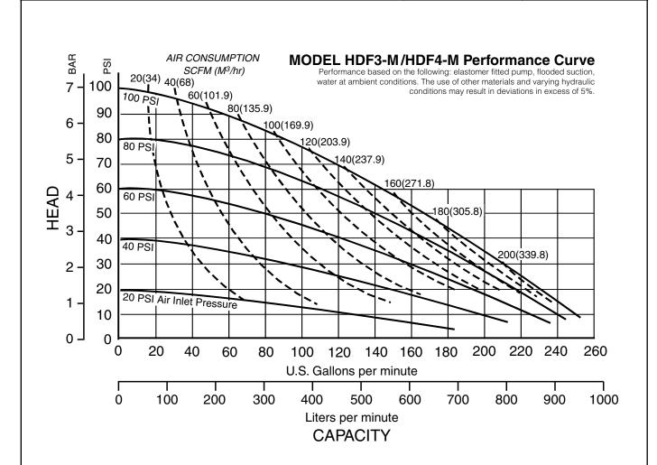
${\bf SANDPIPER}^{\otimes}$  pumps are designed to be powered only by compressed air.
