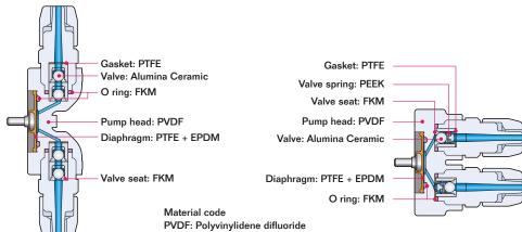
PVDF: Polyvinylidene difluoride FKM: Fluorine-contained rubber PTFE: Polytetrafluoroethylene
