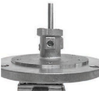
**NOTE:** The setscrew on the seal body should be visible through the 1/8" NPT port.
