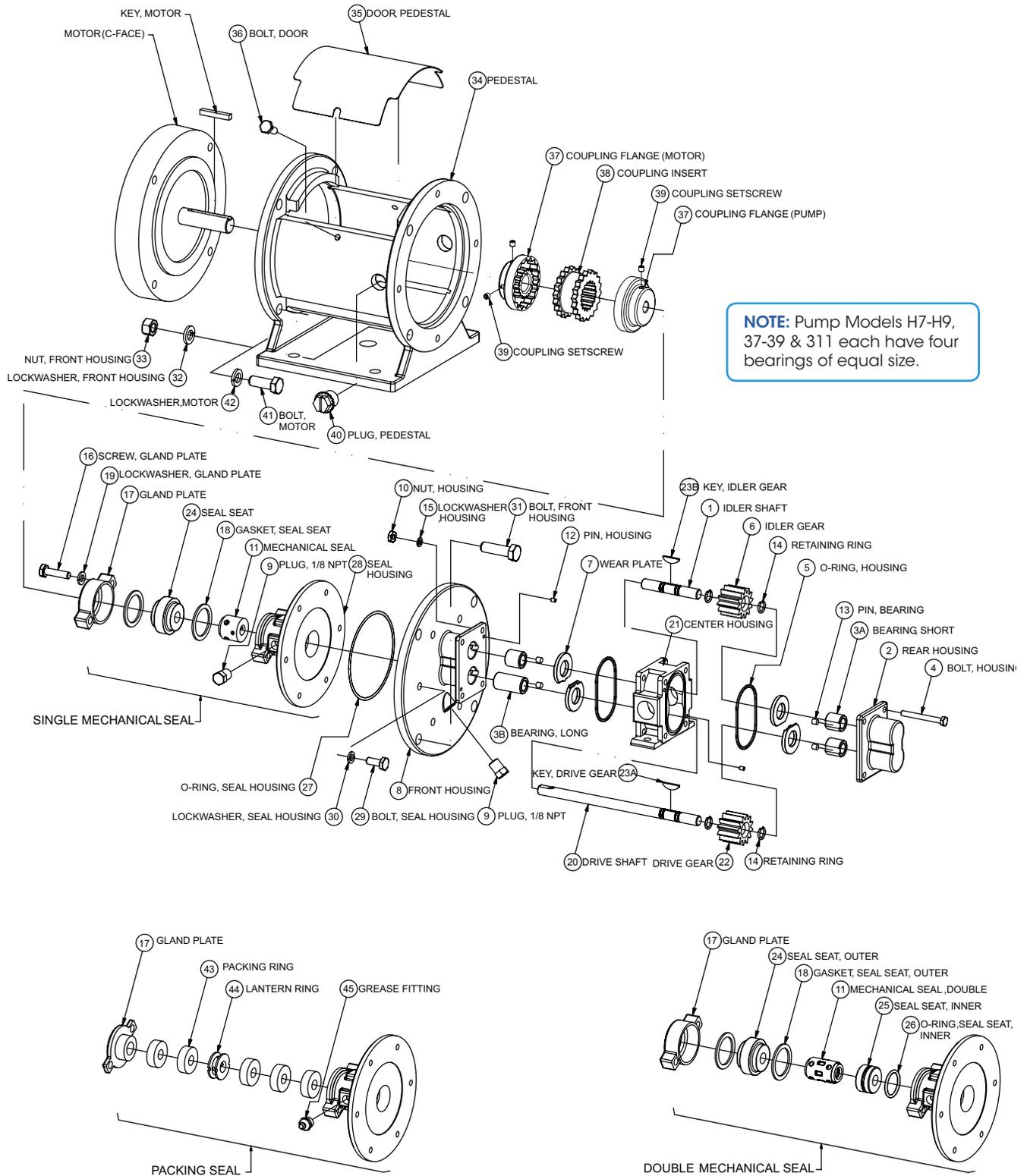
**NOTE:** Pump Models H7-H9, 37-39 & 311 each have four bearings of equal size.
