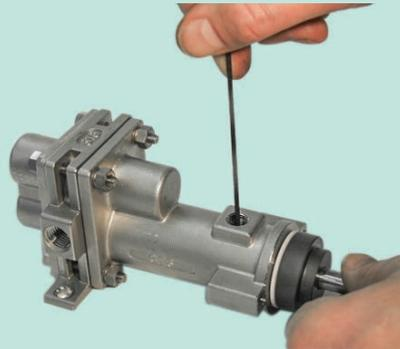
**NOTE:** Rotate the shaft in steps to access each setscrew thru the 1/8" NPT port on the front housing.
