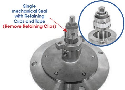
**NOTE:** Do not remove the seal retaining clips until after the seal is installed on the drive shaft.
