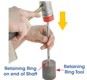
**NOTE:** See Appendix 2 for specifications on producing the retaining ring tool.
