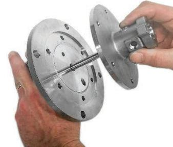
**NOTE:** The seal housing should mate freely with the front housing.
