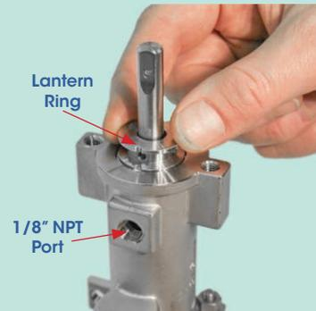
**NOTE:** After installation, the lantern ring should be visible thru the 1/8 inch NPT ports.
