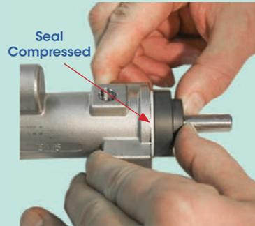
**NOTE:** The outboard seal seat is lapped on both surfaces so orientation does not matter.
