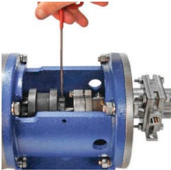
**NOTE:** Tighten only the setscrew on the **flat part of the pump shaft**. This will prevent damaging the round part of the shaft.
