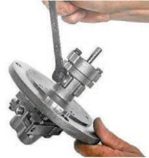
**NOTE:** Apply Teflon tape to the threads of the plug to prevent leakage.
