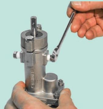
**NOTE:** Apply Teflon tape to the threads of the plugs to prevent leakage.
