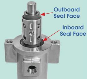
**NOTE:** The double mechanical seal is symmetrical, so the seal faces can be oriented either way.
