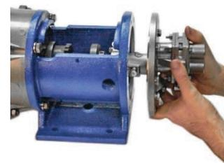
**NOTE:** Ensure that the pump coupling flange mates with the flexible insert.
