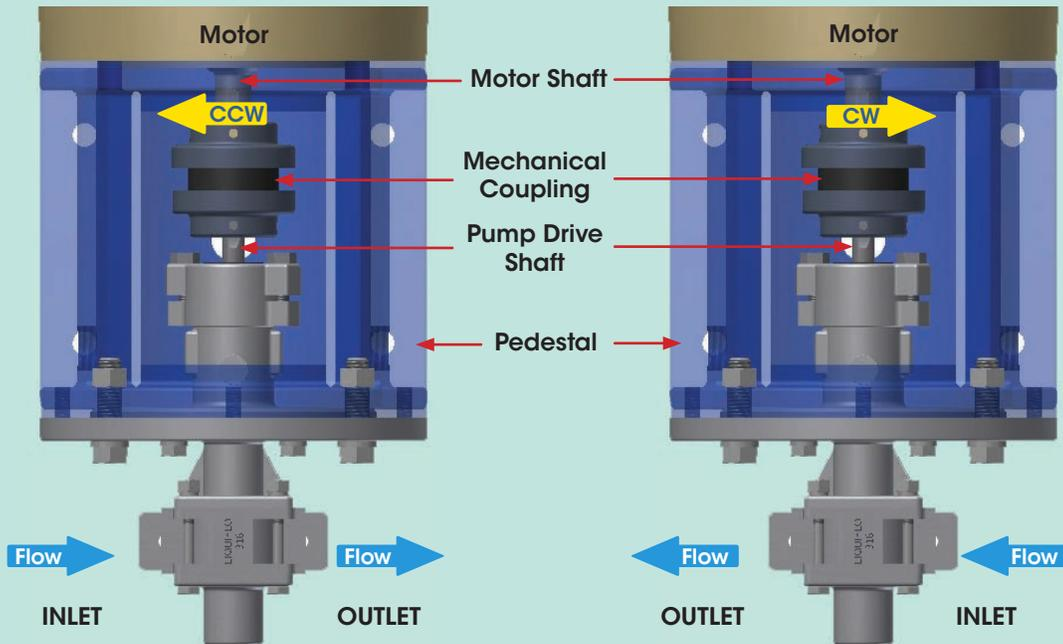
**Counterclockwise (CCW) Rotation of Motor Shaft:**
