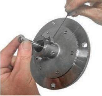
**NOTE:** Rotate the shaft in steps to access each setscrew thru the 1/8" NPT port.
