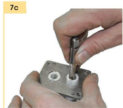
Removal of PEEK or Teflon Bearings
