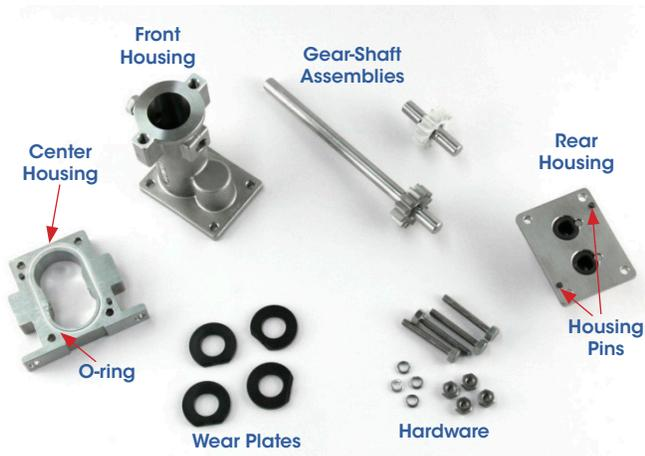
**Gear - Shaft Disassembly:** (If Required; See note above.)
