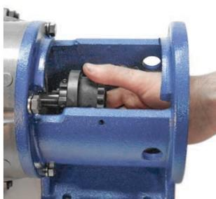
**NOTE:** Do not tighten the coupling setscrew at this time.
