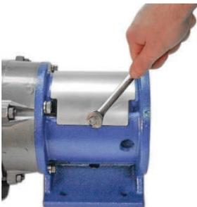
**NOTE:** The door is secured to the pedestal with two bolts on opposite sides.
