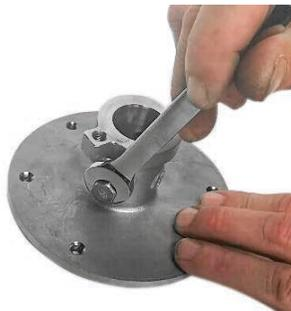
**NOTE:** Apply Teflon tape to the threads of the pug to prevent leakage.
