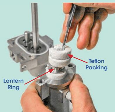
**NOTE:** The packing and lantern ring can be pulled out using a hooked shaped tool.
