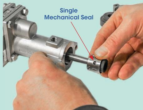
**NOTE:** The setscrews are accessible thru the 1/8" NPT port on the front housing. Rotate the shaft to access the setscrews.
