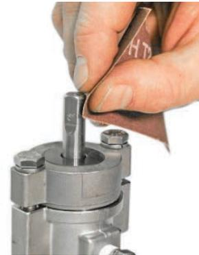
**NOTE:** The round part of the drive shaft may have been scored by the coupling setscrew. If necessary, polish the shaft with fine emery cloth. This will prevent damage to the teflon seal wedge when the mechanical seal is removed or installed on the shaft.
