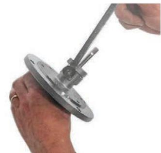
**NOTE:** Remove any burrs or scratches from the end of the drive shaft prior to removing the mechanical seal.
