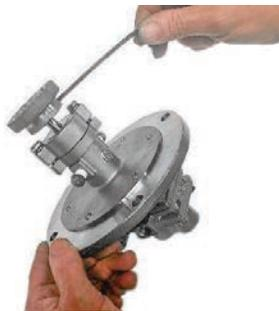
**NOTE:** Tighten the setscrew on the flat part of the shaft **ONLY**. If the coupling has a second setscrew, it should not be tightened. This will prevent damaging the round part of the shaft.
