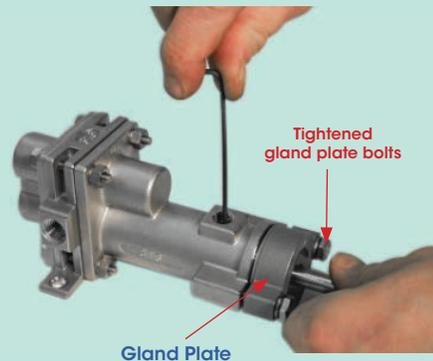
**NOTE:** The outboard seal seat is lapped on both surfaces so orientation does not matter. The double mechanical seal will self-position once the gland plate is installed.
