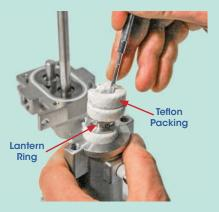
**NOTE:** The packing and lantern ring can be pulled out using a hooked shaped tool.
