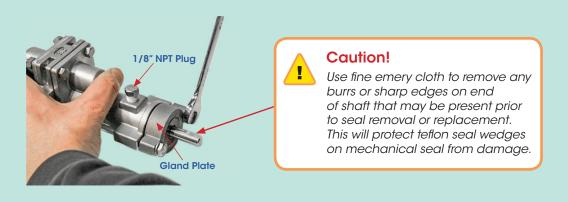
2 Remove the 1/8" NPT Plug (9) then loosen **all** setscrews on the mechanical seal body (11).
