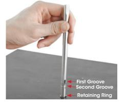
**2 Gentrly** Strike the top end of the shaft with a rubber mallet to force the retaining ring onto the bottom end of the shaft.
