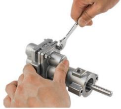
Single mechanical Seal with Retaining Clips and Tape (Remove Retaining Clips)
