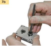
**Removal of Carbon or Sil-carbide Bearings**
