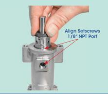
Push the seal into the housing until the setscrew is visible thru the 1/8" NPT port.
