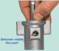
4 Lightly tighten the setscrews on the body of the mechanical seal to temporarily position the seal body.
