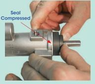
7 Once the position of the mechanical seal is properly set, tighten <u>all</u> setscrews on the seal body.
