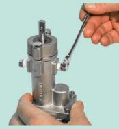
**NOTE:** Apply Teflon tape to the threads of the plugs to prevent leakage.
