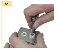
**Removal of PEEK or Teflon Bearings**
