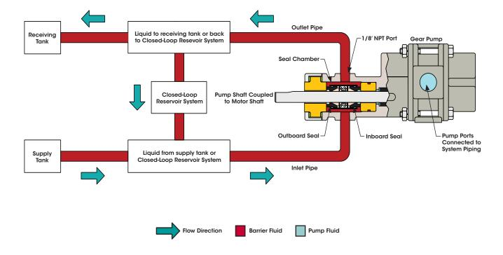
Barrier Fluid Support System for Pump with Double Mechanical Seal
