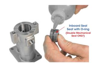
**b)** Insert the inner seal seat (25) into the front housing (8).
