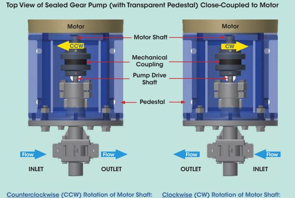
Fluid will enter the pump at the left side (inlet) and be discharged at the **right** side (outlet).
