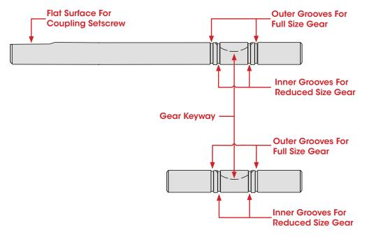
To identify the pump shafts, refer to the following chart:
