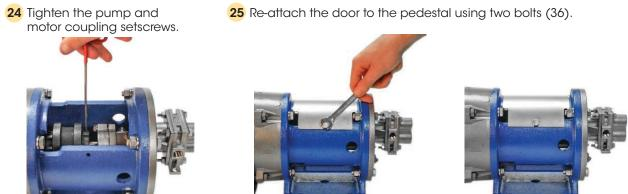
NOTE: Tighten only the setscrew on the flat part of the pump shaft. This will prevent damaging the round part of the shaft.
