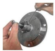
NOTE: Rotate the shaft in steps to access each setscrew thru the 1/8" NPT port.
