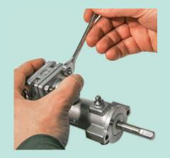
4 Remove the packing (18) and lantern ring (11) from the front housing.
