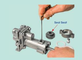
**NOTE:** The setscrews are accessible thru the 1/8" NPT port on the front housing. Rotate the shaft to access the setscrews.
