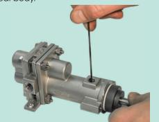
**NOTE:** Rotate the shaft in steps to access each setscrew thru the 1/8" NPT port on the front housing.
