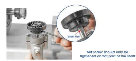
3 Inspect the end of the drive shaft and remove any high spots, scratches or burrs.
