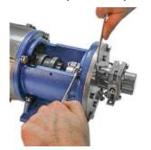
23 Loosen the setscrew on the pump coupling flange and then adjust the position of both flanges so that the flexible insert is free to move axially - a distance of about 1/16 to 1/8 inches.
