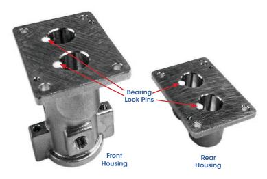
2 Insert the bearings (3A & 3B) into the housing bores. A light push to fit may be required.
