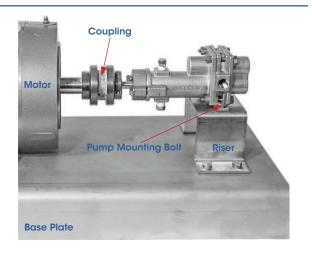
2 Remove the coupling flange from the pump shaft by loosening the setscrew.
