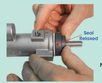
NOTE: The outboard seal seat is lapped on both surfaces so orientation does not matter.
