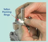
**NOTE:** For teflon rings be sure to stagger the splits in adjacent rings 180° apart.
