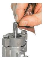
**NOTE:** The round part of the drive shaft may have been scored by the coupling setscrew. If necessary, polish the shaft with fine emery cloth. This will prevent damage to the teflon seal wedge when the mechanical seal is removed or installed on the shaft.
