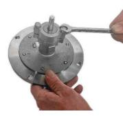
**16** Install the other 1/8" NPT plug (9) into the seal housing (28).
