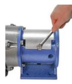
NOTE: The door is secured to the pedestal with two bolts on opposite sides.
