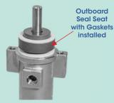
5 First install the gland plate (17) and tighten bolts. <u>Second</u> after the gland plate is installed then tighten <u>all</u> seal setscrews.
