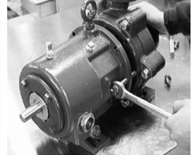
**Fig. 11-4: Jackscrews to Decouple Drives**
