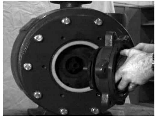
**Figure 9-10 Assembling impeller/rear casing**
