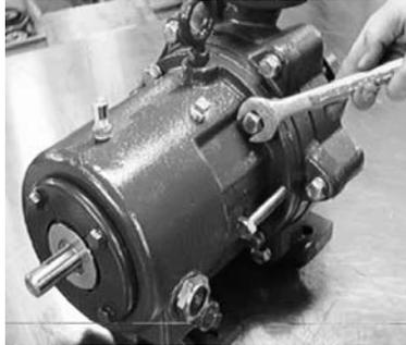
**Fig. 11-3: Bolts to Connect Bearing Frame**
