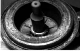
**b)** The rear support is clocked with the two “grooved” ears horizontal. Insert the containment shell into the rear support with the groove in the shaft at the 11:00 O’clock position. If necessary, tap the containment shell into place with a soft hammer until it is evenly seated.
