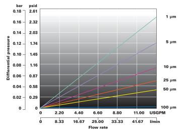
\* For liquids other than water, multiply pressure drop by fluid viscosity in centipoise.
