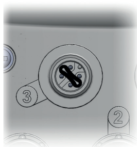
Fig. 9-4: Conductive rubber tube in connection socket 3
