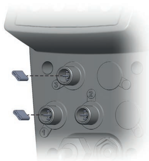
Fig. 9-1: Removing the conductive rubber bands
