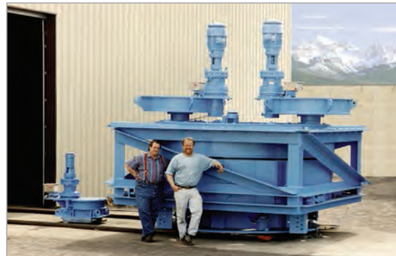
Cage Drive Unit with 2,000,000 ft-lbs torque
