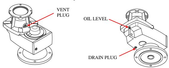
NOTE: For NEMA 250TC and larger standard Perma CLASSIC lubrication system will exist. Please change system according to plug in end of lubricator.
