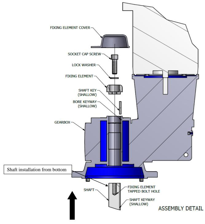
Step 6: (See Bulletin 02-200 for illustration) Remove turbine/turbine hub from packing and slide hub over shaft end until above keyway. Insert key and lower hub into position. Tighten hub set screws into key and shaft.
