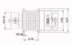
MEMDOS SMART LB 2, 5, 10 with dosing head made of stainless steel 1.4571
