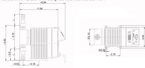
MEMDOS SMART LB 15, 20 with dosing head made of PVC, PP, PVDF or stainless steel 1.4571
