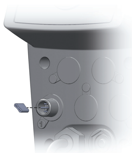
Fig. 27: Removing the conductive rubber band
