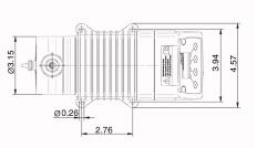
MEMDOS SMART LK 2, 5, 10 with dosing head made of stainless steel 1.4571
