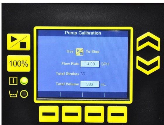
Figure 26: Pump Calibration (Start Flow)
