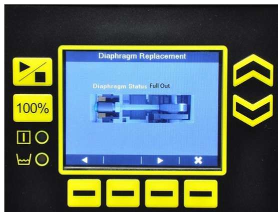
Figure 30: Diaphragm Replacement (Full Out)
