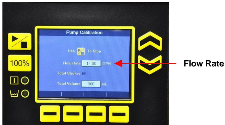
Figure 25: Pump Calibration (Set Flow Rate)
