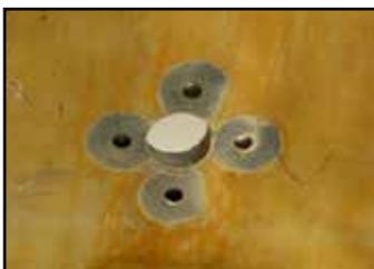
**Fitting and Outlet Chemical Exposure** – Since it is difficult to mold a uniform wall of linear polyethylene within the dual layered tank processing technique, fitting locations often have to be ground down and smoothed over to achieve a uniform sealing surface, which can inevitably result in the removal of the linear layer and the required chemical resistance protection that goes with it.
