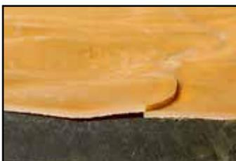
**Delamination** – Linear polyethylene is a thermoform plastic, which means it can be melted and cured multiple times. Crosslinked polyethylene is a thermoset plastic, which means the cure is permanent, and cannot be reset. The two plastics do not permanently bond. In application, the sidewall expansion and contraction caused by a tank being filled and emptied creates further long-term stress on the two materials' seam. As a result, end users have experienced delamination failures.
